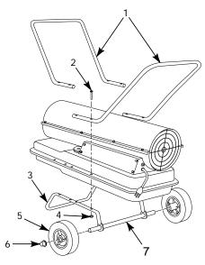
Figure 25 - Handle and Wheel Assembly
